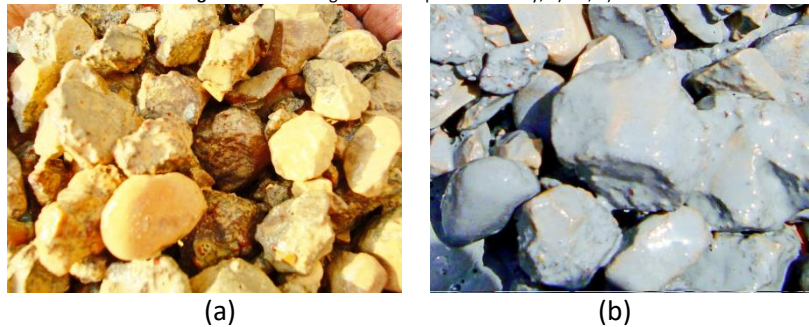
Figure 5. Presoaking of RCCA in pozzolan slurry; a) NZ, b) SF.
