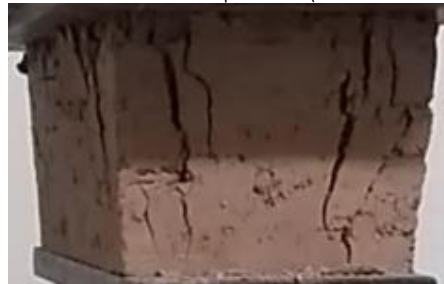
Figure 4. Failure mechanism in sample control (Source: Self-elaboration).
