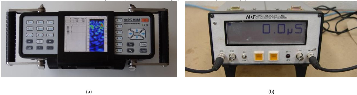
Figure 1. (a) 3D Ultrasonic Tomographer and (b) UPV portable equipment.
