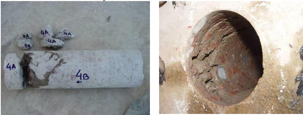
Figure 13. Visual examination of extracted cores in the structure B.
