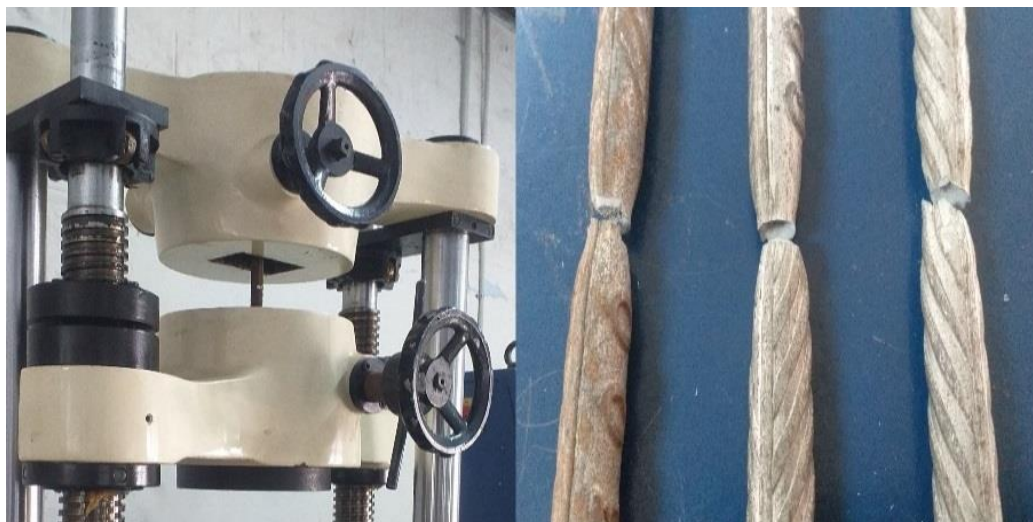
Figure 3. Tensile test on steel rebars.
