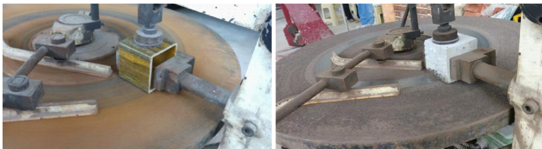
Figure 6. GFRP box profile and concrete wear tests.
