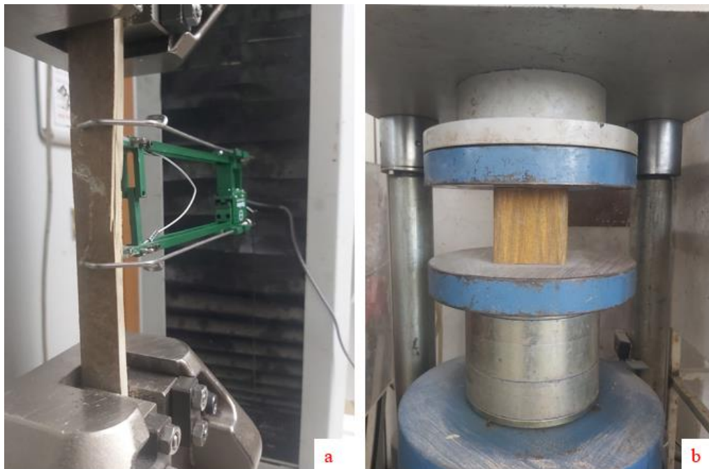
Figure 4. a) Tensile, and b) compressive test sample.
