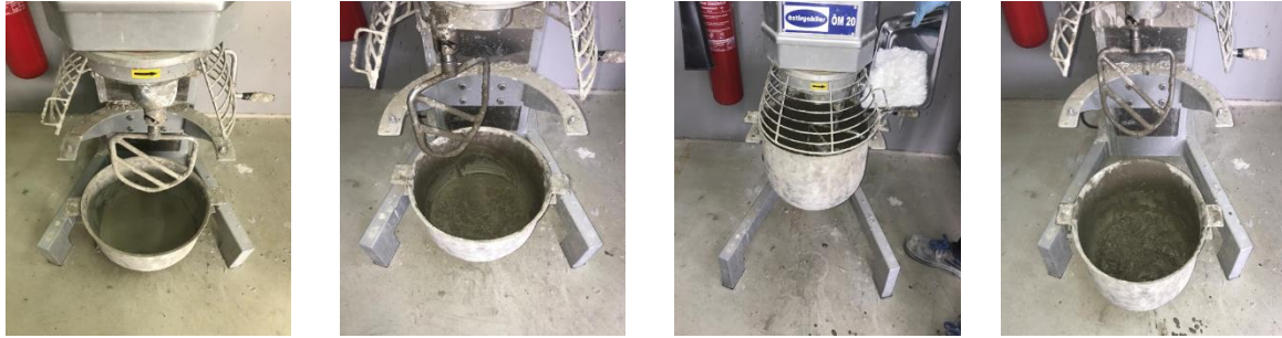
Figure 2. Production of ECC mixtures.
