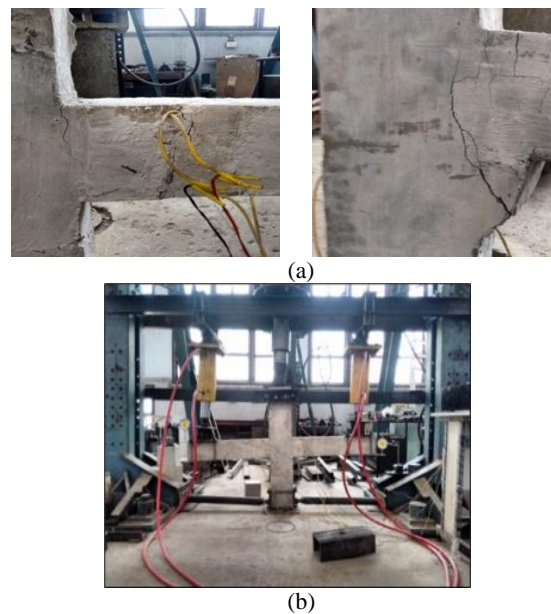
Figure 7. (a) Damages observed in the MBC-EJ and EBC-EJ Specimen, (b) relative rotation between the beams and column of MBC-IJ specimen observed during experimentation.
