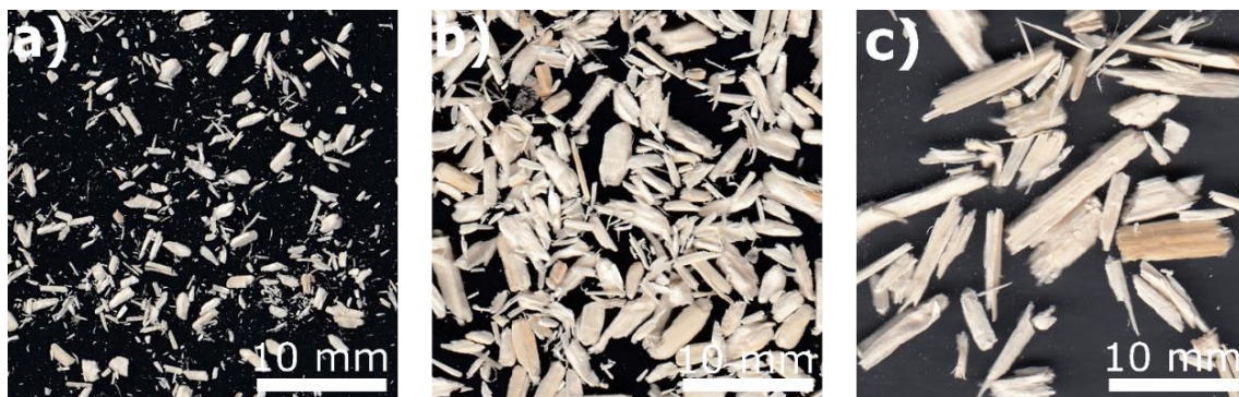
Figure 3. Hemp shivs used in the study a) fine, b) medium, and c) coarse.
