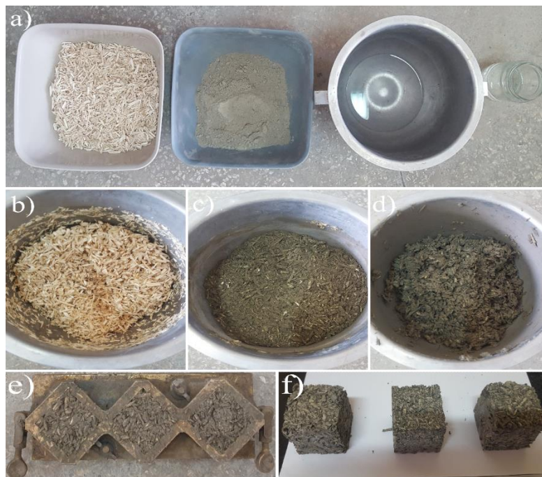
Figure 6. Preparation of hemp composite samples: a) weighted materials for mixture, b) hemp shiv mixed with 65% of mixing water, c) after addition of chosen cement amount, d) after mixing with the rest of water, e) casted samples in cubic molds, f) Casted samples named HC4HW3C.
