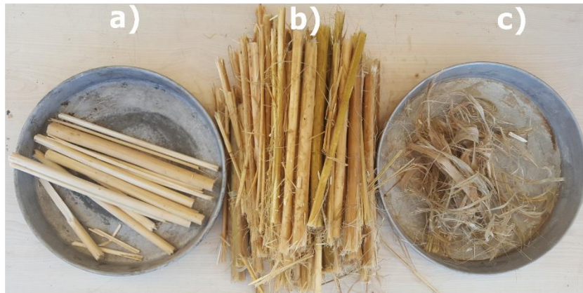
Figure 2. The process of obtaining bare hemp stems: a) hemp stems without fibers, b) hemp stems kept in water filled container for 21 days, and c) hemp fibers removed from the stems.
