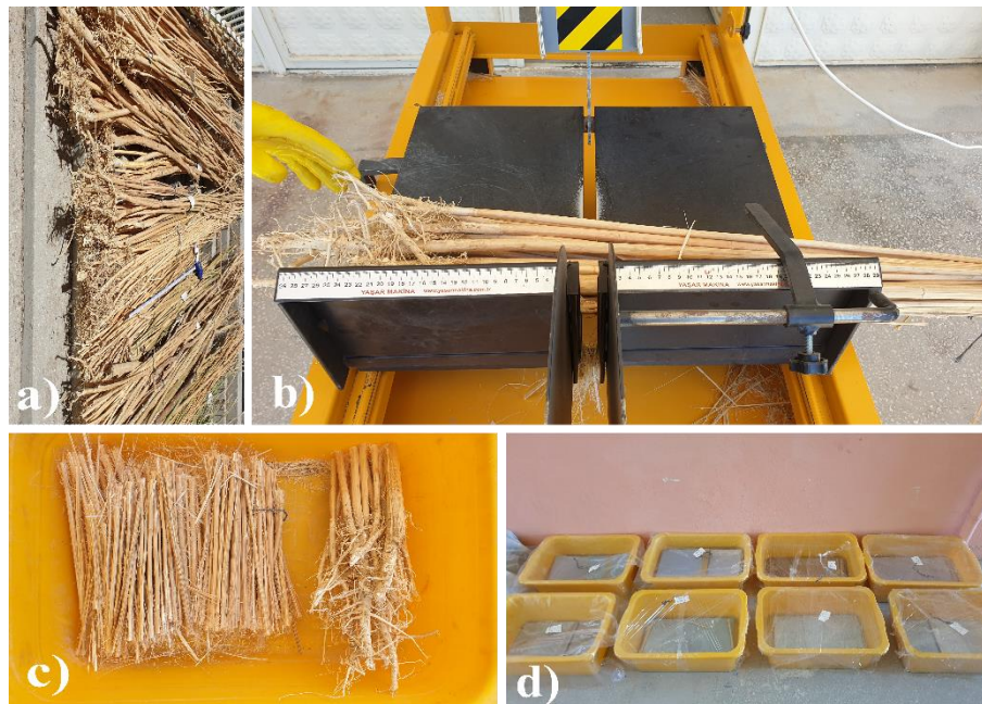
Figure 1. Retting process of hemp stems: a) Industrial hemp stems with various lengths, b) Sawing hemp stems in pieces of ~30 cm, c) Sawed hemp stems in container before retting, d) Retting of hemp stems in the water filled container.
