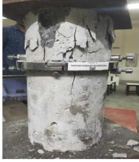
Figure 7. Crushing of cylinder specimen.
