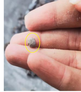
Figure 8. WAP balls shrinks and forms a hard cement product.
