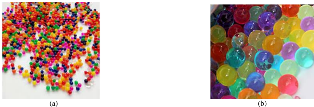
Figure 1. Water absorption polymer balls: (a) dry polymer balls (b) water absorbed polymer balls.
