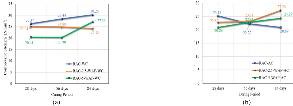
Figure 5. Compressive strength of recycled aggregate concrete with and without WAP balls (a) water cured specimen (b) air cured specimen.
