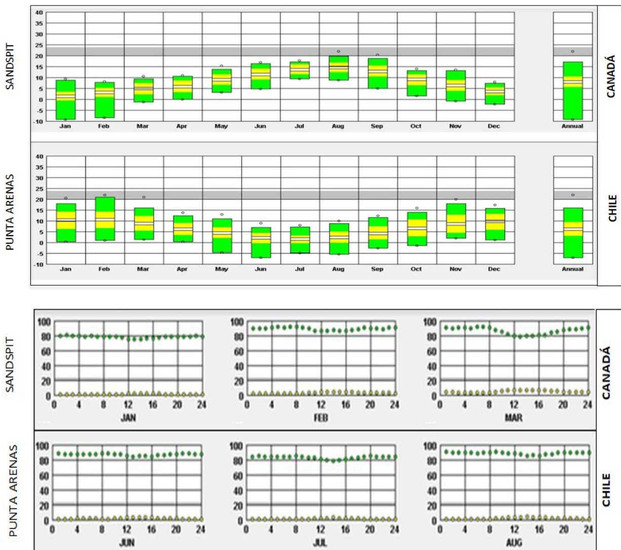
Figure 1. Temperature and humidity comparison diagram obtained using Climate Consultant. Source: Climate Consultant, using weather files in Energy Plus Weather format (.epw)
