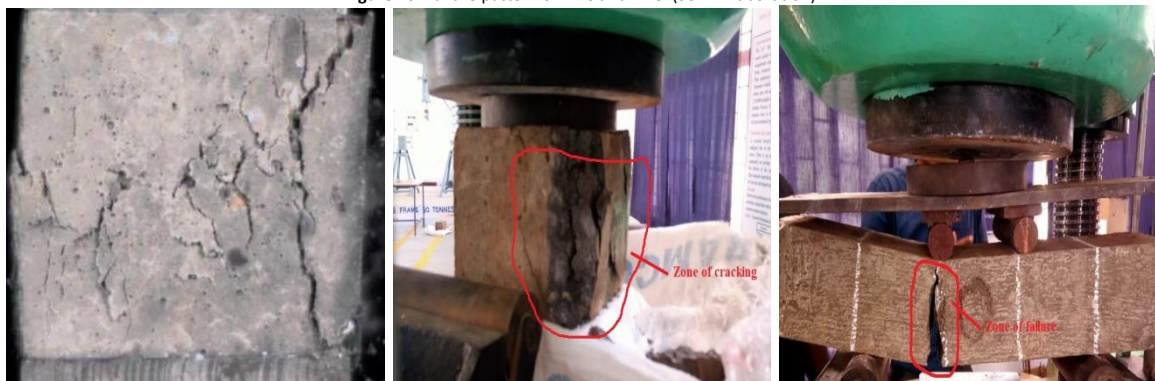
Figure 10. Failure pattern of NAC and RAC. (Self – Elaboration).
