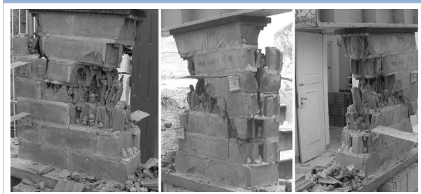
Figure 2. Compression tested brickwork specimens, made with A manufacturer's perforated bricks. Source: Self-elaboration, 2014.
