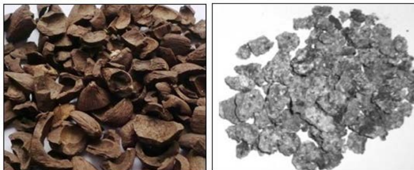
Figure 1: Coarse aggregate (A) OPS aggregate (B) POC aggregate. Source: Self-Elaboration.
