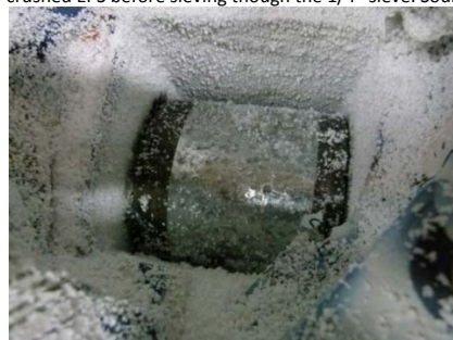
Figure 1. Aspect of crushed EPS before sieving though the 1/4" sieve. Source: Self-elaboration.
