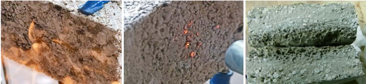
Figure 4. Direct flame test process and final aspect of the sample of dimensions 24x12x5cm. Source: Self-elaboration.
