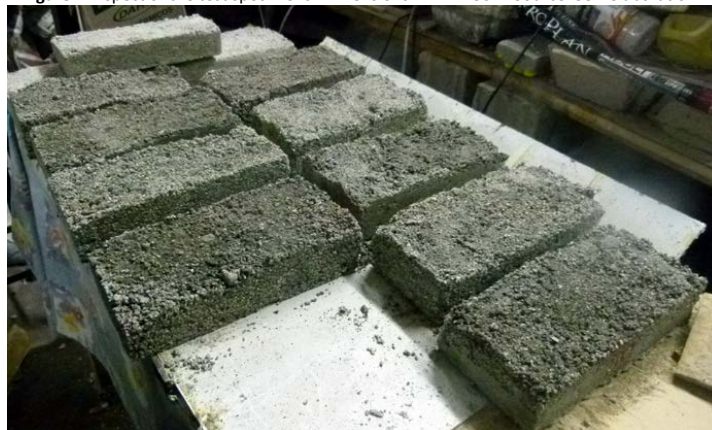
Figure 2. Aspect of the test specimens: Dimensions: 24x12x5cm. Source: Self-elaboration.
