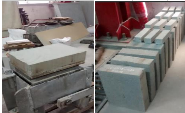
Figure 5. Raw-perlite bricks produced with a CINVA RAM hand press. Source: by the author.
