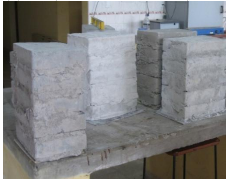
Figure 13. Masonry specimens produced with a CINVA RAM hand press. Source:by the author.
