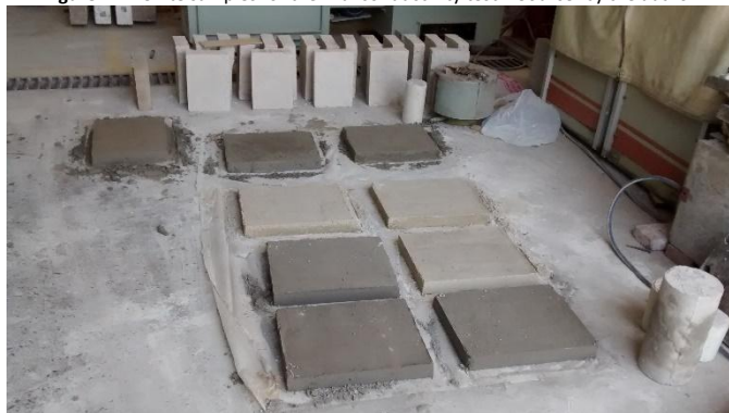
Figure 12. Perlite samples for thermal conductivity test. . Source: by the author.
