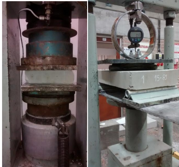
Figure 7. Compressive test (left) – Flexion text (right). Source: by the author.
